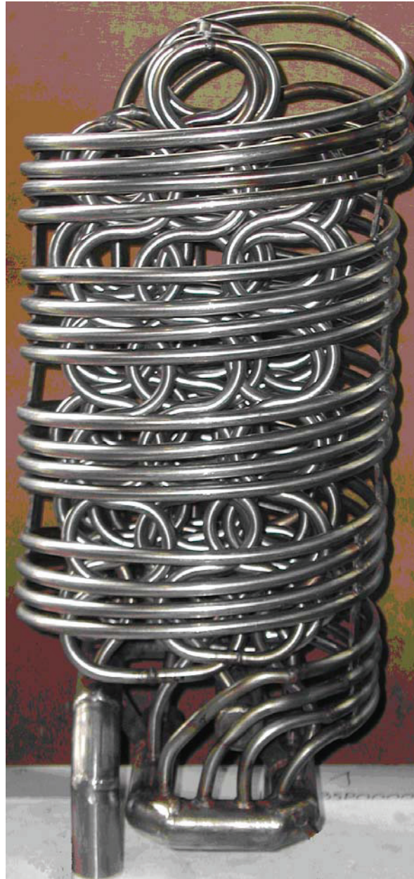
Fig. 7.3: SFBC-EFMGT fluidized bed heat exchanger prototype 1
