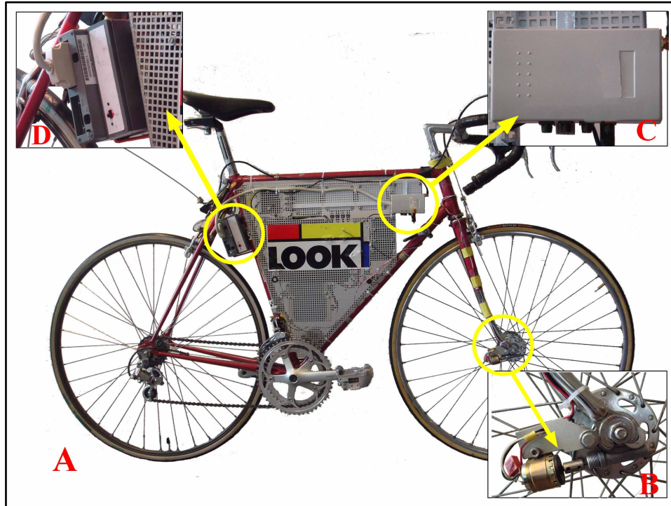
Figure 7 Illustration of (A) telemetry-bicycle system consists of (B) a tachogenerator (speed sensor), (C) a connector box, and (D) a transmitter unit with an antenna.
