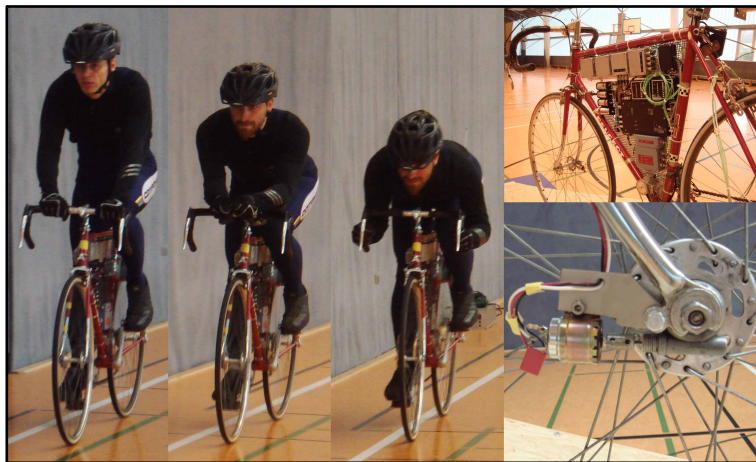
Figure 4.2 Illustrations of upright position (UP), aero position (AP), and fully dropped position (DP) during the coasting down test. A tachogenerator, equipped on a distal of the front fork of the bicycle, was used to measure the velocity-time function through a telemetry bicycle, which transmitted a signal at 433.92 MHz to a receiver module.
