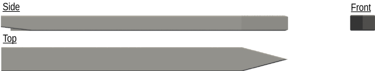
Figure 5.2: Top, side and front views over the generic hull form
