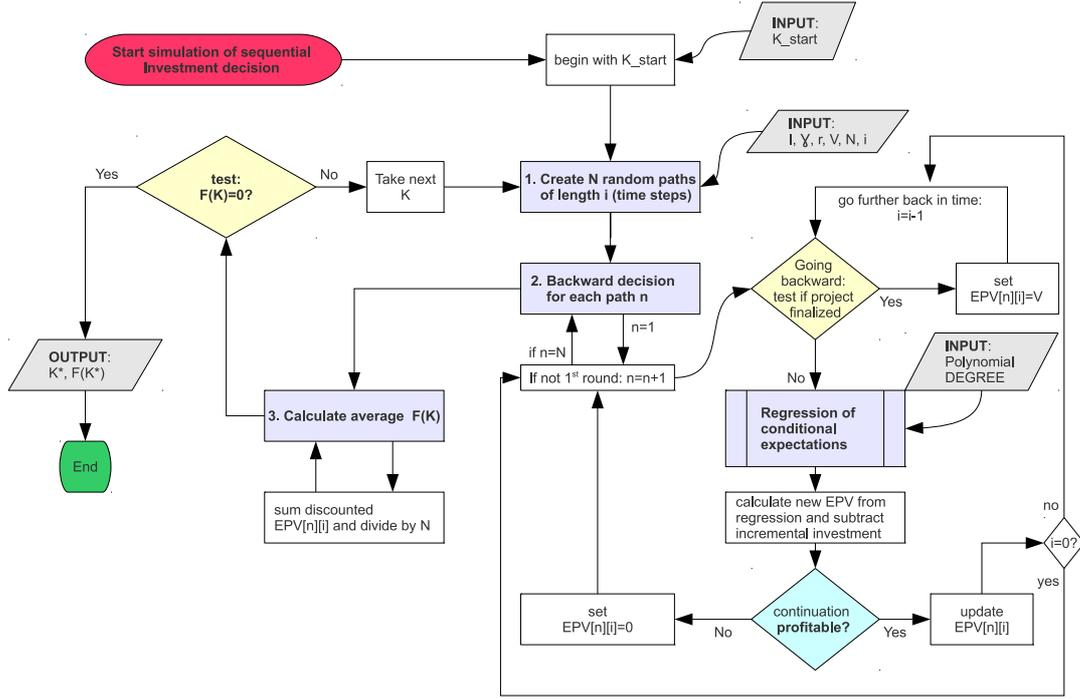
Figure 3.3.: Flow chart of the Monte Carlo code to solve the basic sequential investment model under technical uncertainty.
