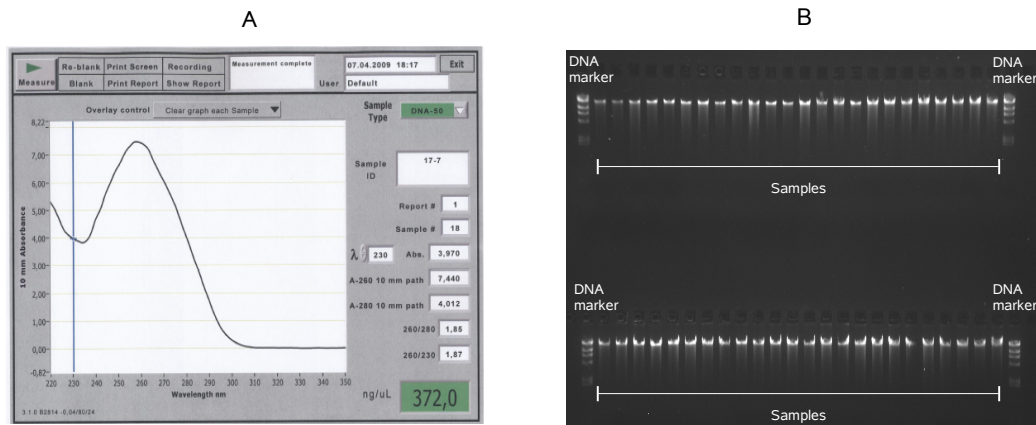
Figure 2.2: An example for each quality and quantity test for DNA. A graphical output from the NanoDrop 1000 Spectrophotometer (A). A picture taken after the gel electrophoresis (B).
