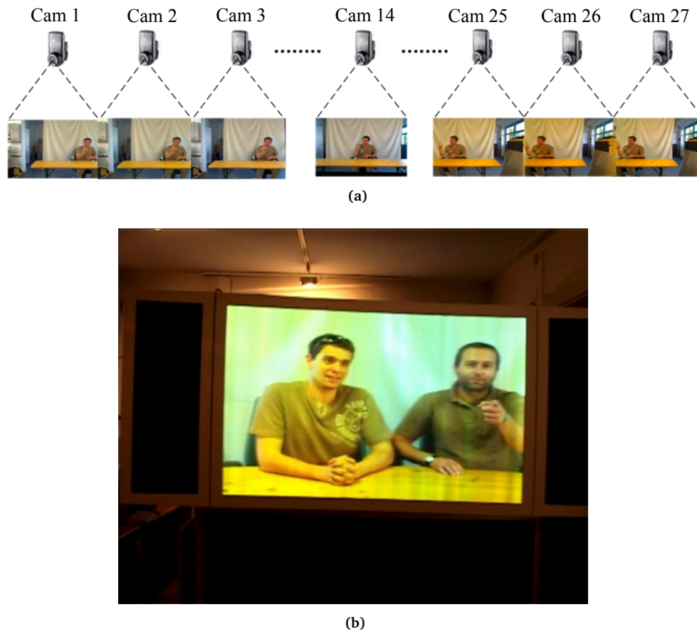
Figure 5.12 – Sample scene acquisition and reconstruction for light field display: (a) sample light field capturing, (b) light field reconstruction.
