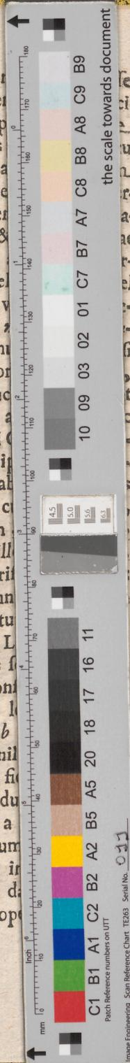
Image Engineering Scan Reference Chart TE36.1 Serial No. 0111
