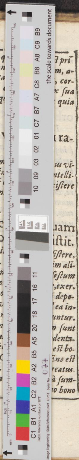
Image Engineering Scan Reference Chart TE263 Serial No. 1234567890
