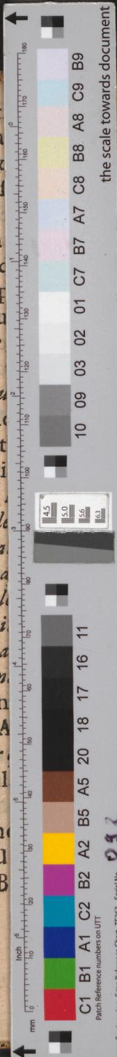
Image Engineering Scan Reference Chart TE63 Serial No. 033
