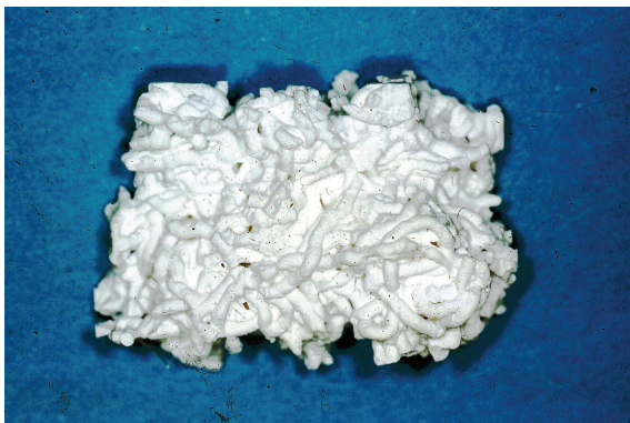
Figure 4.3: View from the ready for implantation material (BCP silica-based ceramic) in form of “spaghetti”
