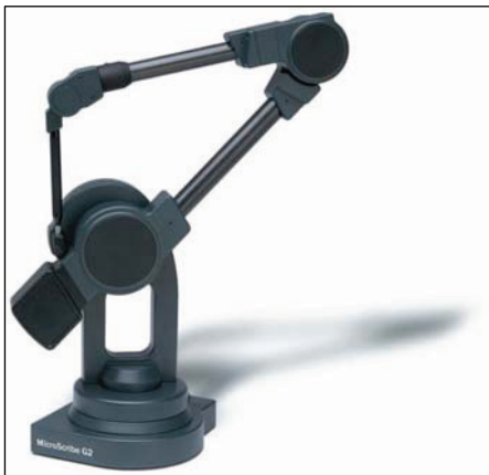
Abb. 6: MicroScribe G2 3 D Digitizer der Firma Immersion Corporation (US), aus http://www.immersion.com/digitizer/products/microscribe_g2.php
