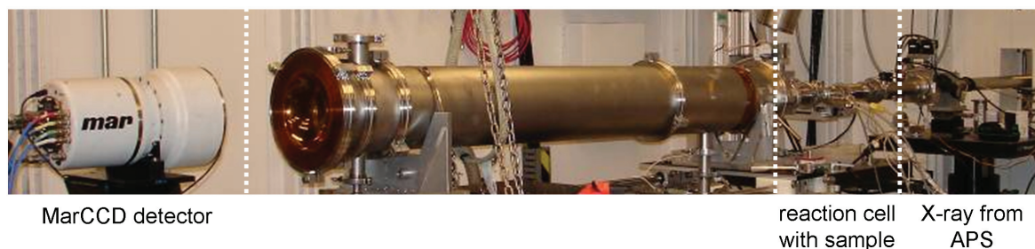
Figure 3.13.: Experiment setup at the 12-ID beamline at the Advanced Photon Source (Argonne National Laboratory). The beam enters from the right into the reaction cell, where the interaction with sample takes place. The detector on the left is used to record the scattering image.
