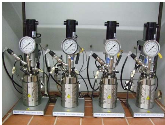
Fig. App. 1(b). Photographs of autoclaves used for oxidation reactions.
