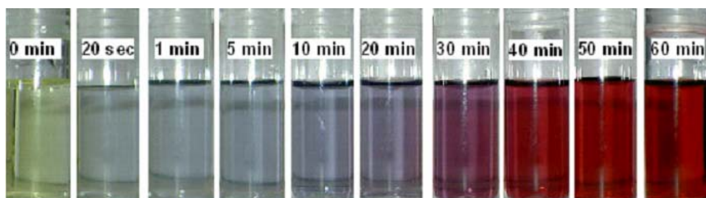
Fig. 3.13. Color changes of the reaction solution during the course of colloidal AuNPs formation with SC as reducing agent.
