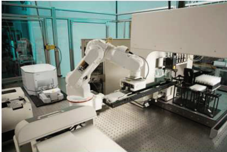
Figure 13 Articulated 6-axis robot in lab automation work cell, source: Beckman Coulter, Inc.
