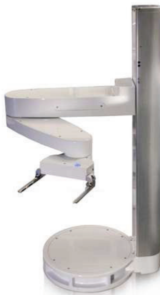
Figure 14 Scara robot 'direct drive robot', source: Agilent Automation
