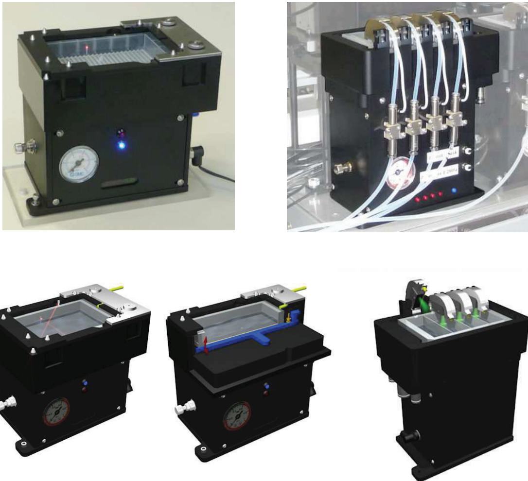
Figure 65 Self Refilling reservoirs, photographs and CAD studies
