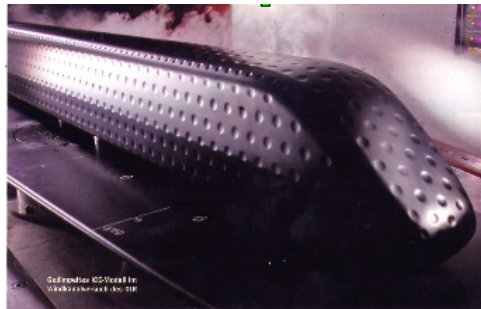
Fig. 1.2: Application of dimples on ICE trains to reduce side drag [100].
