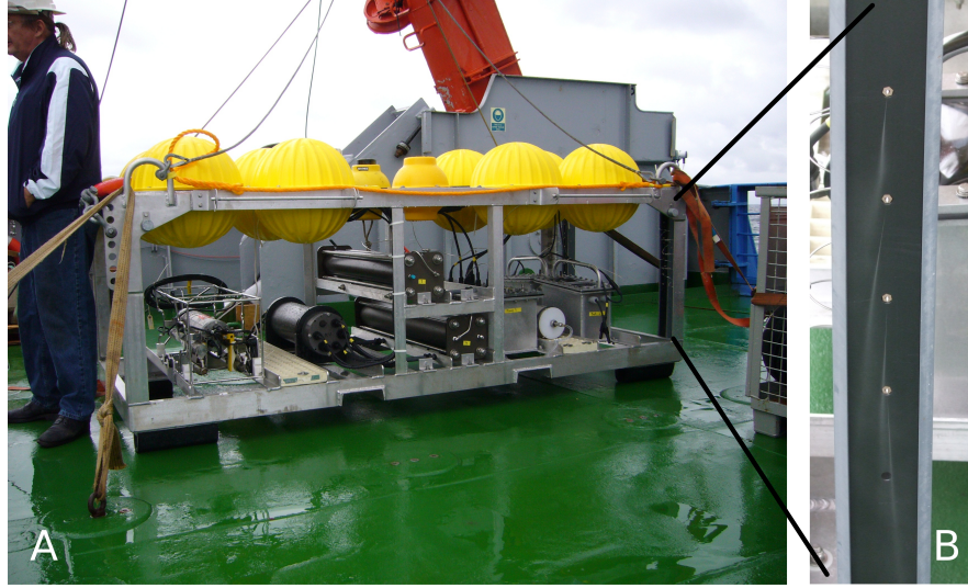
Figure 3.2.: The Ocean Tracer Injection System, OTIS, (a) on board of the RV Poseidon September 2007. Zoom on the injection orificies (b).
