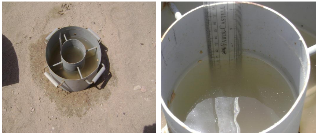
Figure (App.2.5): The double-rings infiltrometer device used to perform the infiltration test.
