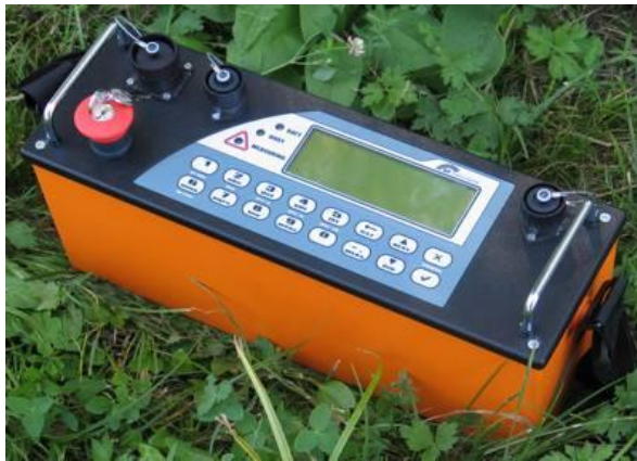
Figure (5.9): The geo-electric measuring device (Automatic resistivity meter, ARES).
