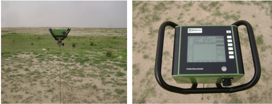
Figure (App.2.6): The Penetrometer device used to perform the penetration test at Jleep Landfill.
