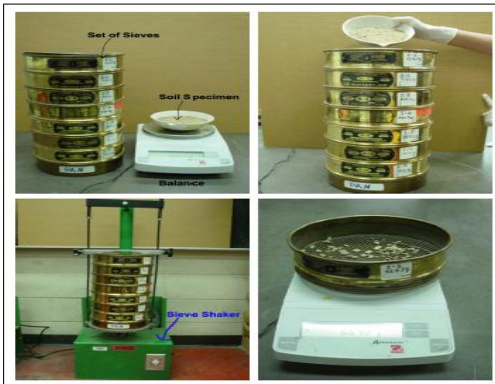
Figure (App.2.4): Equipment used for the determination of grain size percent distribution is samples collected from the covering layer in Jleeb landfill site.
