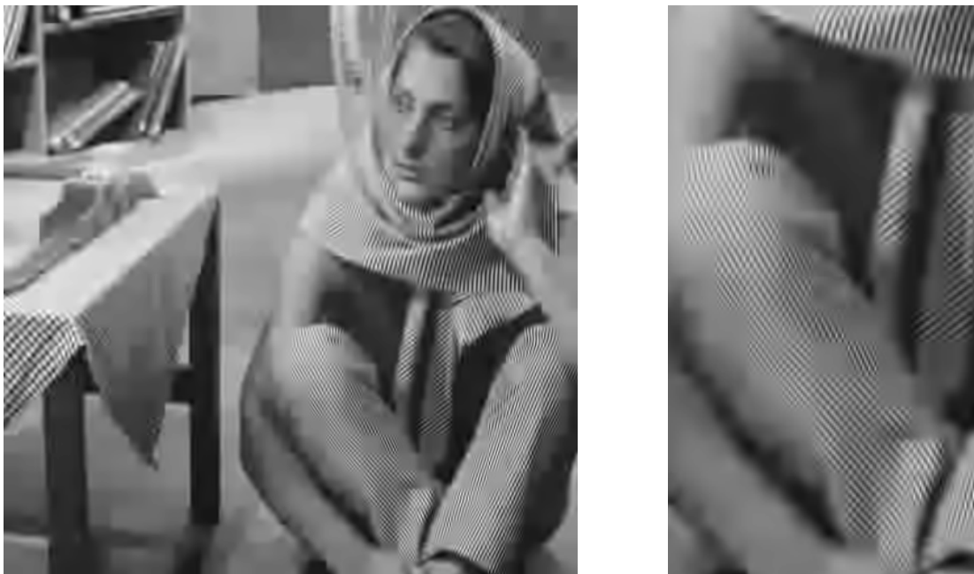
Abbildung H.169: AGU-Codec-II pp, 16 \times 16 DCT & 2-level DWT, PSNR = 25.67 dB.
