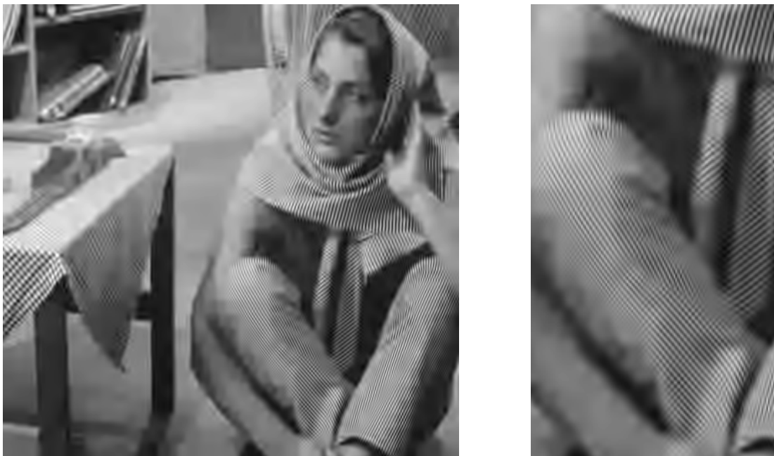
Abbildung H.193: AGU-Codec-II pp, 16 \times 32 LCT-2 & 2-level DWT, PSNR = 26.49 dB.
