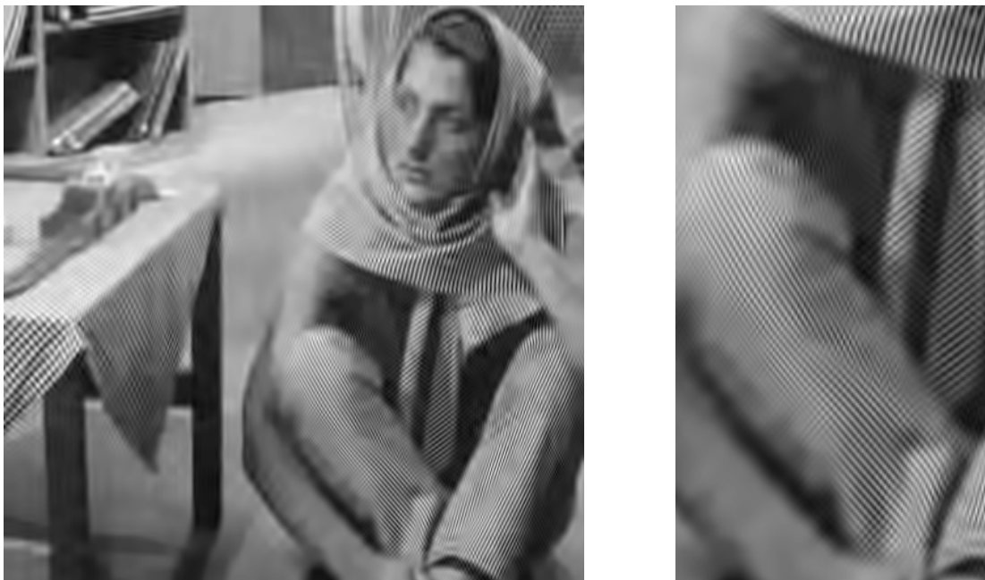
Abbildung H.197: SPIHT-Codex-II pp, 32 \times 64 LCT-2 & 1-level DWT, PSNR = 26.30 dB.
