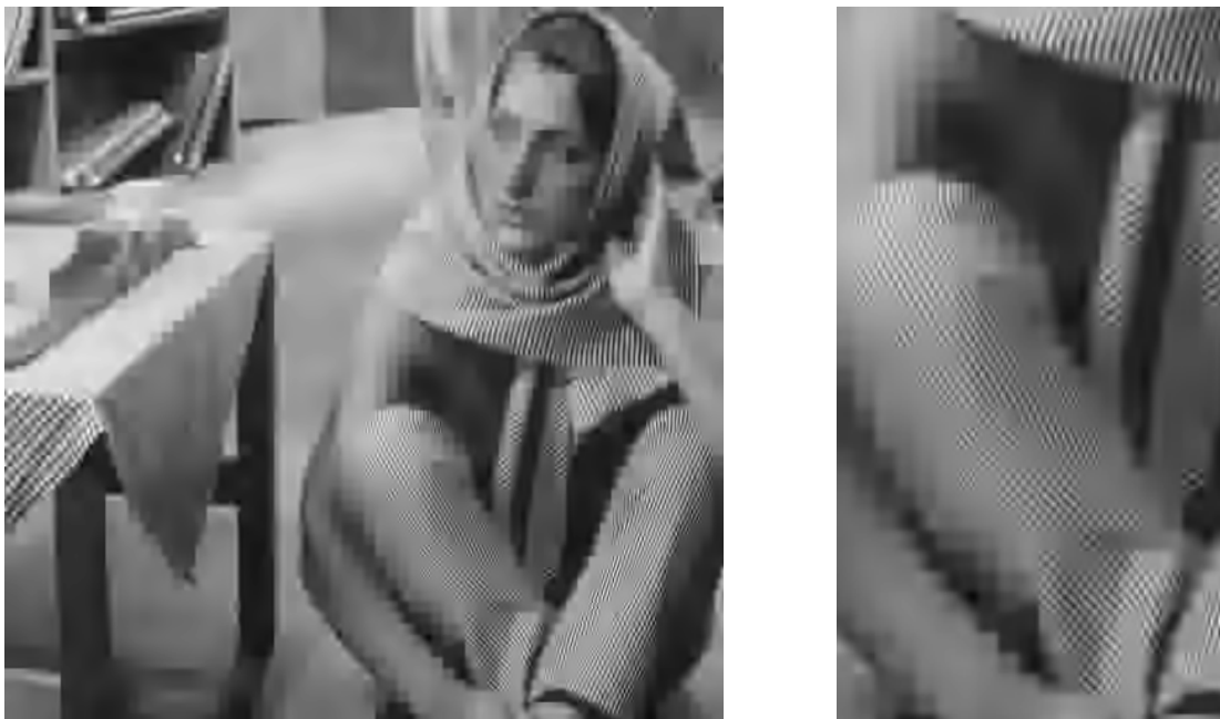
Abbildung H.161: SPIHT-Codec-II pp, 8 \times 8 DCT & 3-level DWT, PSNR = 24.61 dB.
