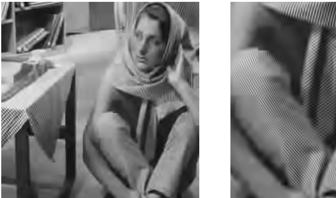
Abbildung H.173: SPIHT-Codec-II pp, 32 \times 32 DCT & 1-level DWT, PSNR = 25.77 dB.
