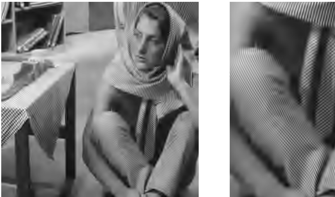
Abbildung H.221: L-CEB-Codec-II pp, 8 \times 32 LCT-4 & 3-level DWT, PSNR = 26.38 dB.
