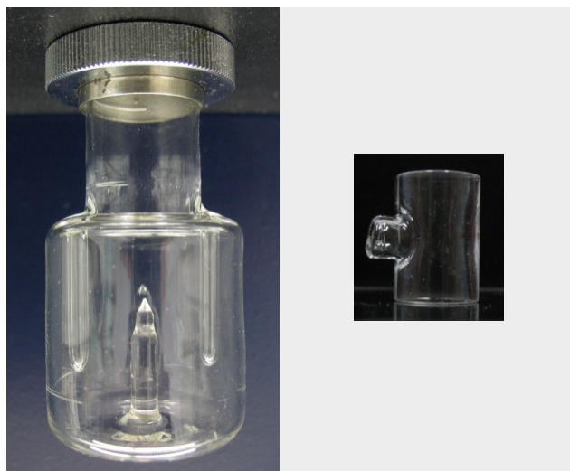
Figure 6.4. Calorimetric cell and crushing ampoule
