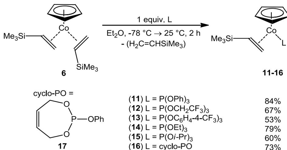
**Scheme 11:** Synthesis of mixed CpCo(I)-olefin-phosphite complexes
