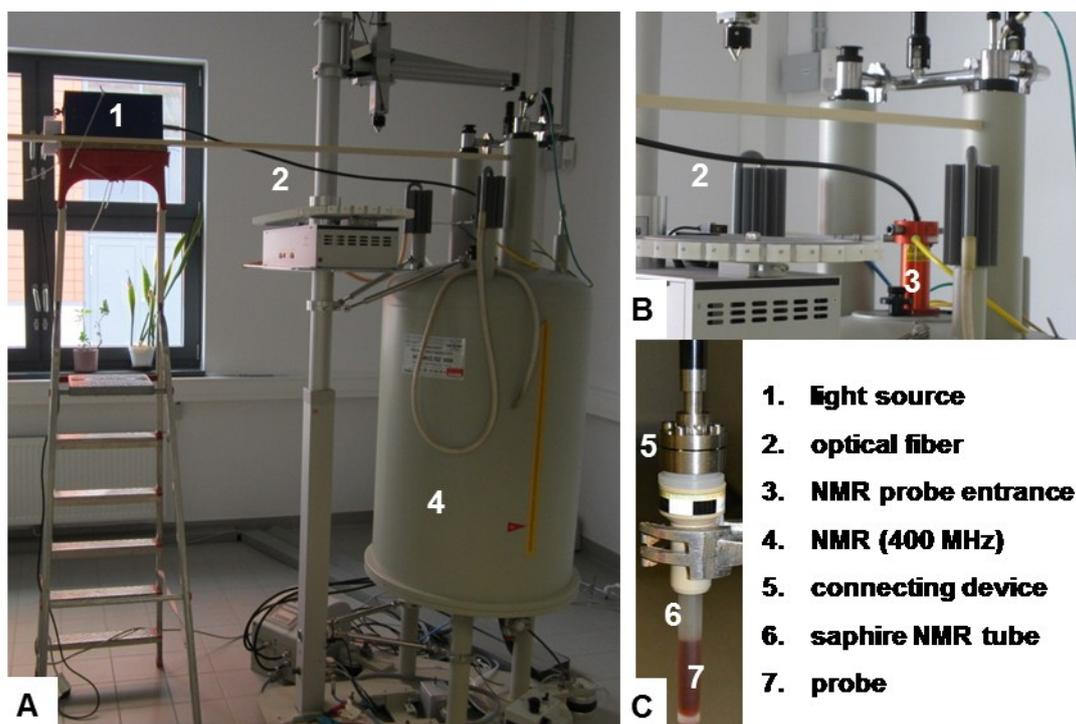
**Figure 14:** Experimental setup for the *in situ* NMR spectroscopy; **A:** optical fiber connecting NMR spectrometer with the light source; **B:** close-up of the entrance of the NMR; **C:** custom-made NMR tube with reaction mixture and connected optical fiber
