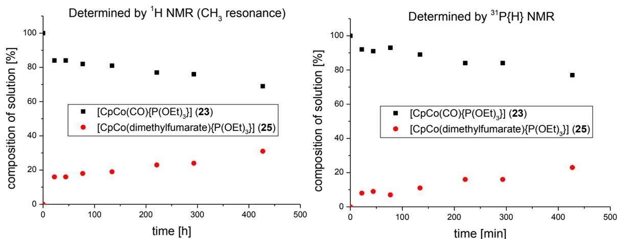
**Figure 18:** Composition of the reactant solution determined by  $^1\text{H}$  NMR using the  $\text{CH}_3$  resonance of the coordinated and free dimethylfumarate (left) and by  $^{31}\text{P}\{\text{H}\}$  NMR (right)
