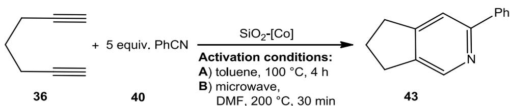
**Scheme 43:** Catalytic test reaction between 1,6-heptadiyne (**36**) and benzonitrile (**40**)
