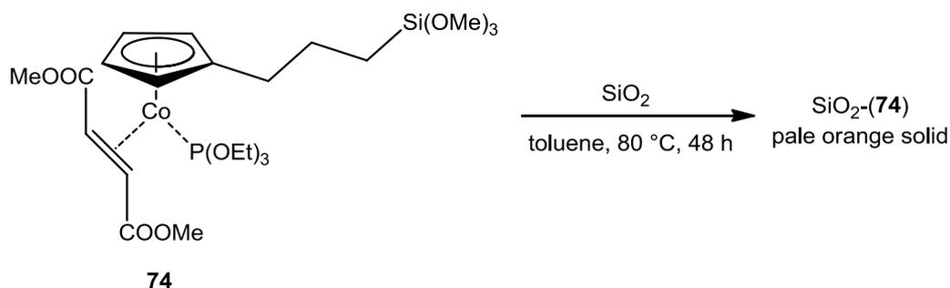
**Scheme 42:** Synthesis of silica-supported  $\text{SiO}_2\text{-}(\mathbf{74})$
