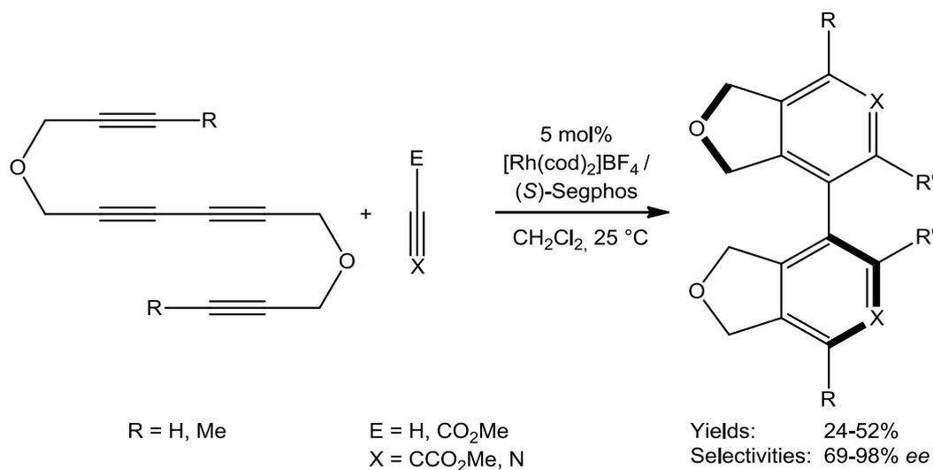
**Scheme 7:** Synthesis of axially chiral biaryls and bipyridines
