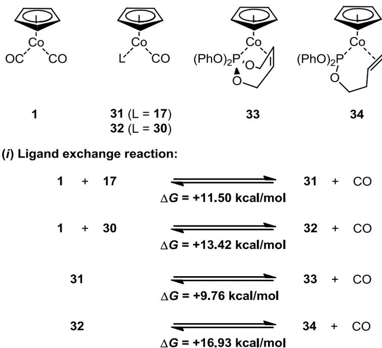
**Scheme 29:** Calculations on the formation of the new complexes **31-34** from **1**, **17** and **30** at BP86/TZVP level
