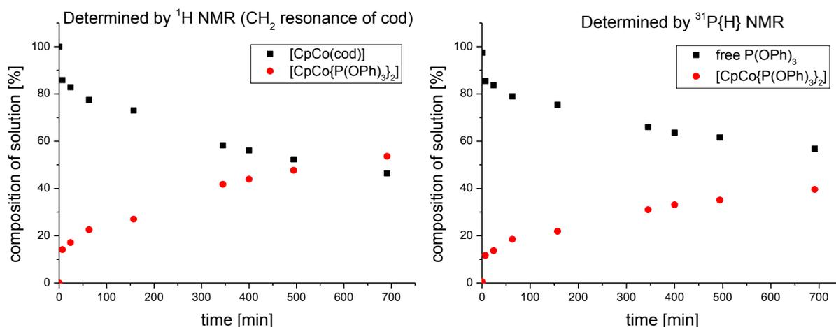
**Figure 16:** Composition of the reactant solution determined by  $^1\text{H}$  NMR using the  $\text{CH}_2$  resonance of the coordinated and free cod (left) and by  $^{31}\text{P}\{\text{H}\}$  NMR (right)
