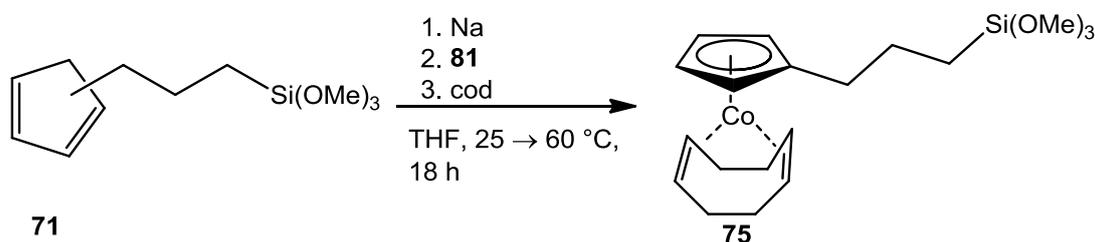
**Scheme 38:** Synthesis of  $[\text{Cp}^{\text{Si}}\text{Co}(\text{cod})]$  complex **75**
