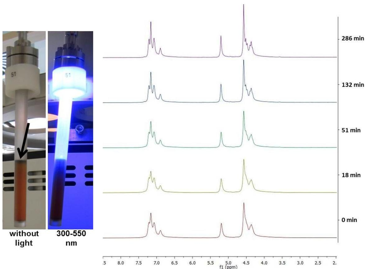
**Figure 19:** Left: custom-made NMR tube with reaction mixture after irradiation (arrow indicates the black pellet of decomposition products at the surface of the solution); right: overlay of the recorded  $^1\text{H}$  NMR spectra of **31**
