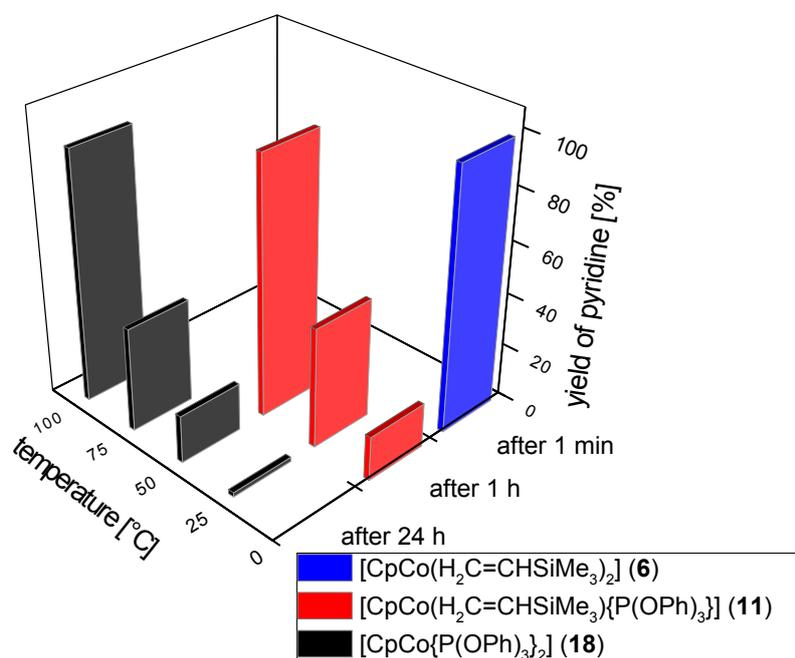
**Figure 13:** Temperature-dependent yields of pyridine (**43**) determined for [CpCo(H<sub>2</sub>C=CHSiMe<sub>3</sub>)<sub>2</sub>] (**6**, blue), [CpCo(H<sub>2</sub>C=CHSiMe<sub>3</sub>){P(OPh)<sub>3</sub>}] (**11**, red) and [CpCo{P(OPh)<sub>3</sub>}<sub>2</sub>] (**18**, black), respectively
