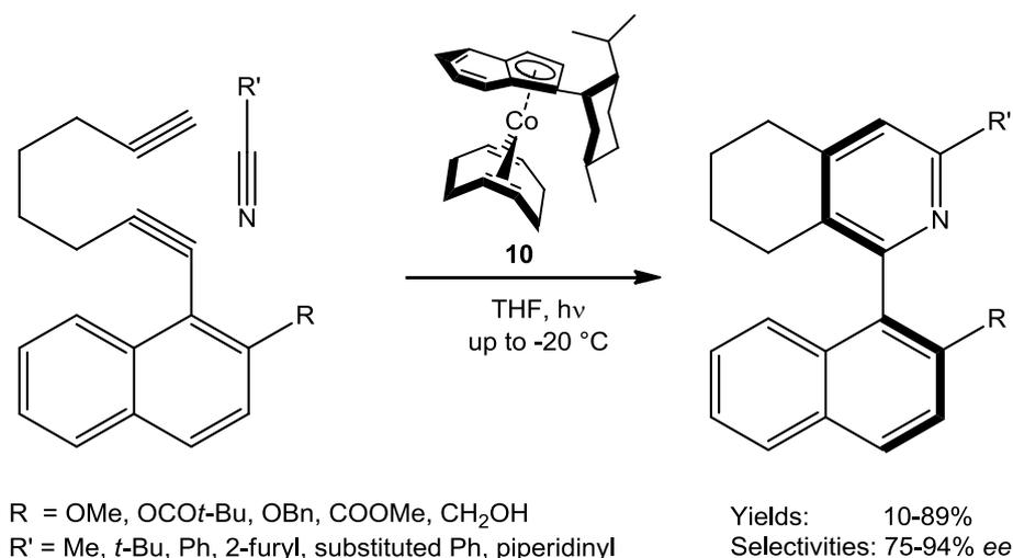
**Scheme 8:** Application of a chiral Co(I)-catalyst in the synthesis of biaryls
