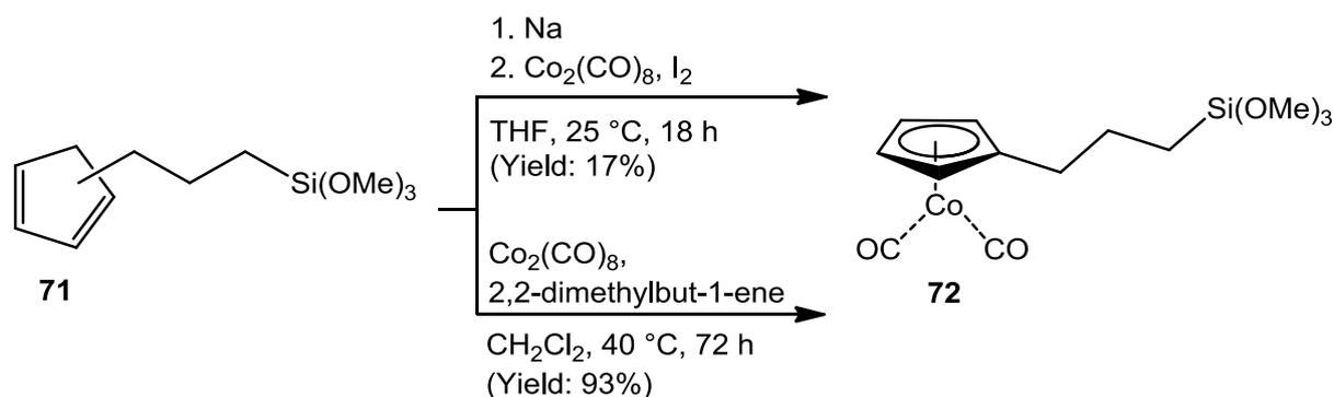
**Scheme 36:** Synthesis of  $[\text{Cp}^{\text{Si}}\text{Co}(\text{CO})_2]$  (**72**)
