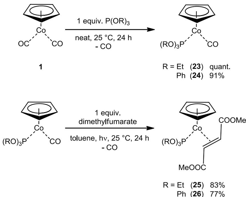
**Scheme 14:** Synthesis of air-stable CpCo(I)-olefin-phosphite complexes
