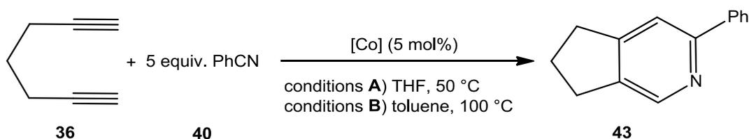
**Scheme 19:** Catalytic test reaction between 1,6-heptadiyne (**36**) and benzonitrile (**40**)
