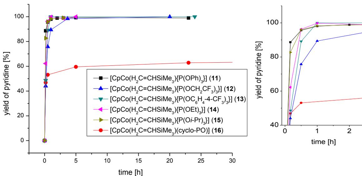
**Figure 4:** Catalytic activity of **11-16** (condition A, Scheme 19) (right: excerpt of the initial phase)
