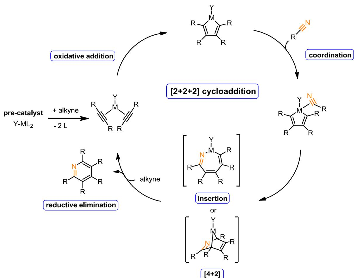
**Scheme 2:** Mechanism of the transition metal-catalyzed [2+2+2] cycloaddition (Y: steering ligand; M: metal; L: neutral ligand)
