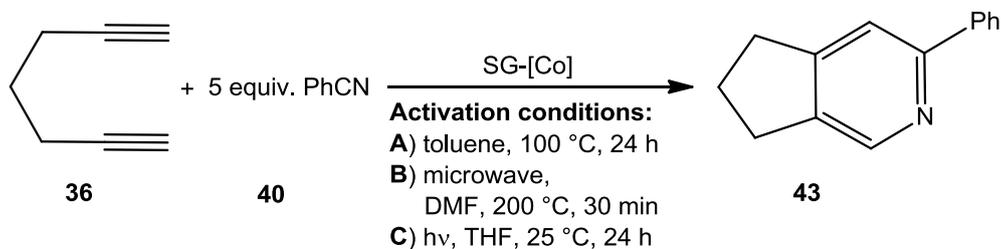
**Scheme 40:** Catalytic test reaction between 1,6-heptadiyne (**36**) and benzonitrile (**40**)
