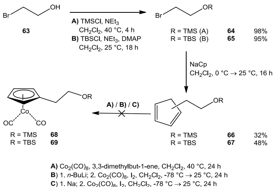
**Scheme 34:** Synthesis of substituted cyclopentadiene derivatives and attempted synthesis of  $\text{Cp}^{\text{OR}}\text{Co}(\text{CO})_2$  complexes
