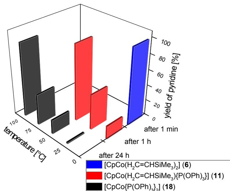
**Scheme 52:** Temperature-dependent yields of pyridine (**43**) determined for [CpCo(H<sub>2</sub>C=CHSiMe<sub>3</sub>)<sub>2</sub>] (**6**, blue), [CpCo(H<sub>2</sub>C=CHSiMe<sub>3</sub>){P(OPh)<sub>3</sub>}] (**11**, red) and [CpCo{P(OPh)<sub>3</sub>}<sub>2</sub>] (**18**, black), respectively
