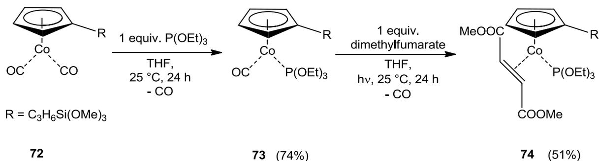
**Scheme 37:** Substitution of the CO ligands in  $[\text{Cp}^{\text{Si}}\text{Co}(\text{CO})_2]$  (**72**)
