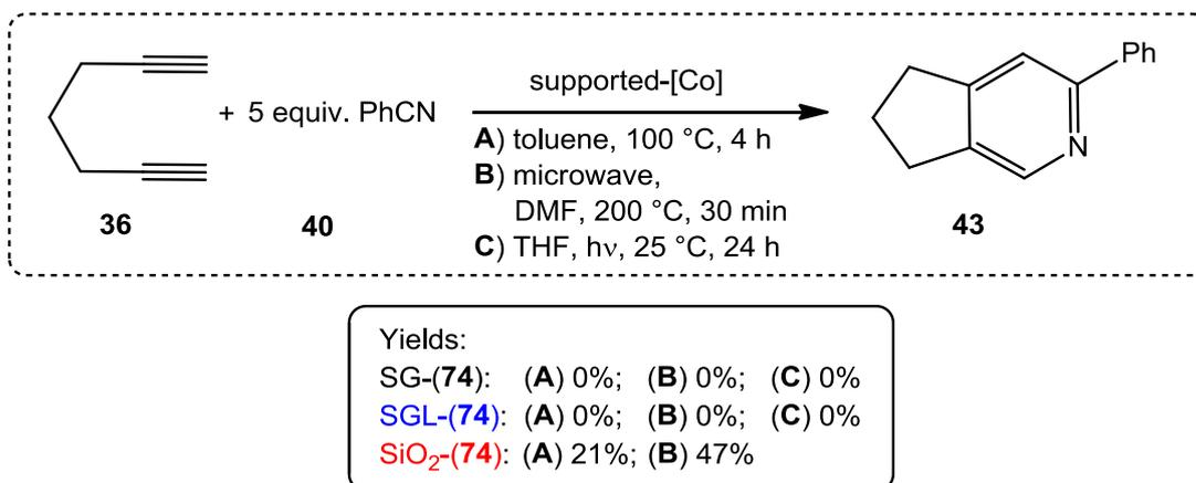
**Scheme 54:** First solid-supported CpCo(I)-catalyst active in the synthesis of pyridines
