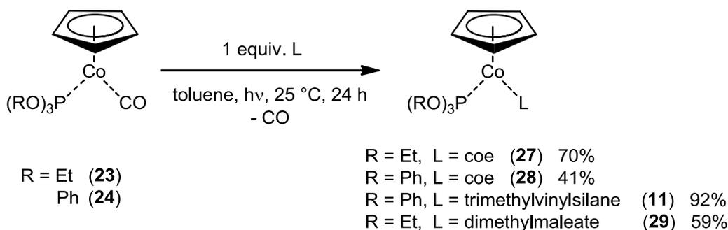
**Scheme 16:** Synthesis of CpCo(I)-olefin-phosphite complexes with varying olefins
