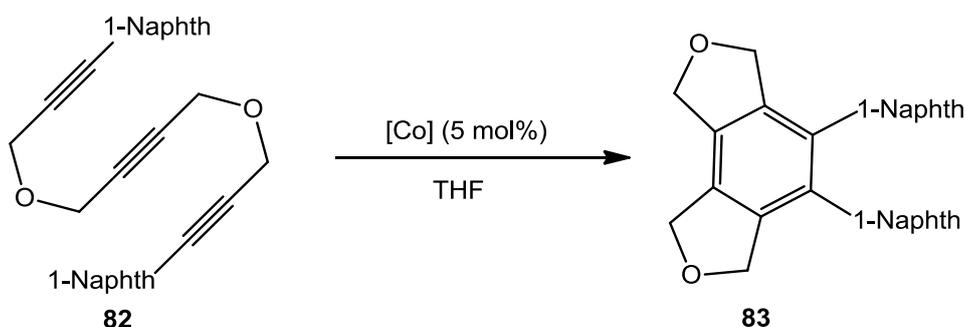
**Scheme 48:** Test reaction for the *in situ*-generated chiral catalysts
