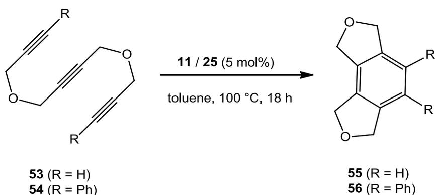
Scheme 22: Substrate screening conditions for **11** and **25**Table 3: Substrate screening for **11** and **25**
