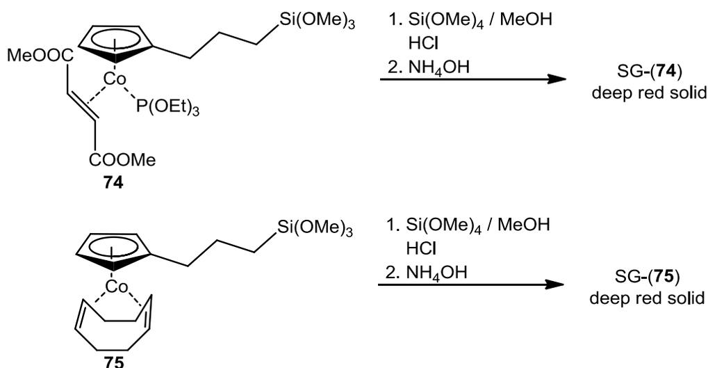
**Scheme 39:** Synthesis of sol-gel-supported SG-(74) and SG-(75)
