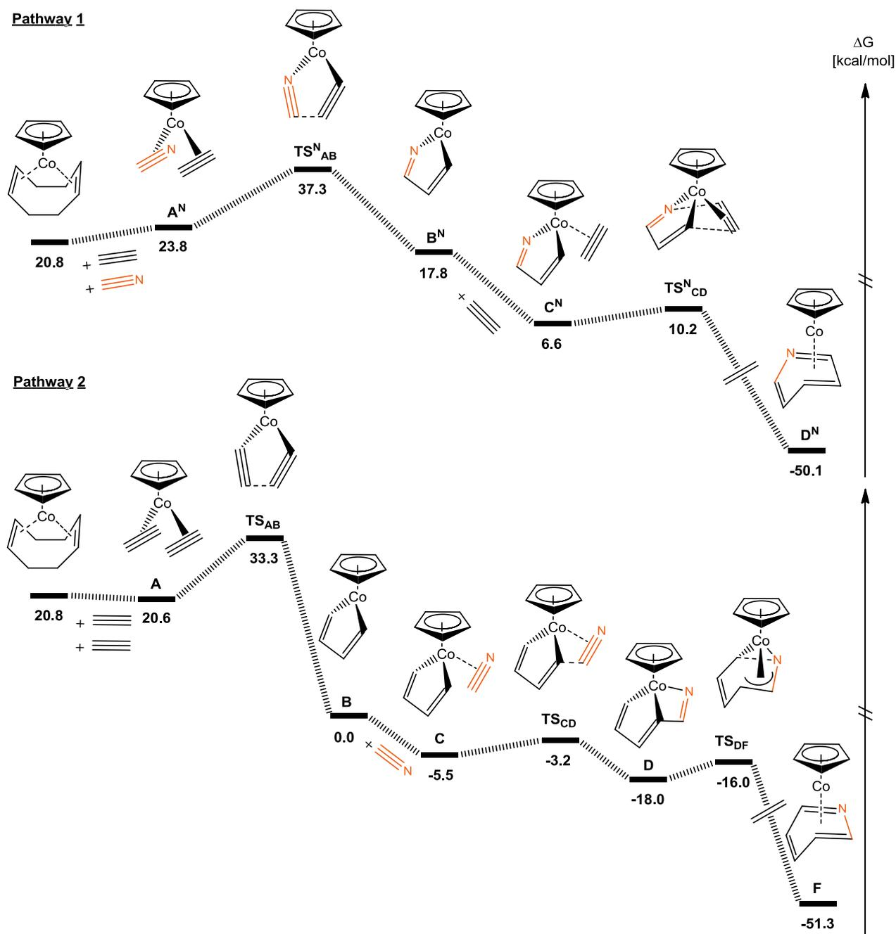
**Scheme 3:** Free energy profiles (in kcal mol<sup>-1</sup>) for the different coordination sequences in the [2+2+2] cycloaddition reaction between acetylene and hydrogen cyanide
