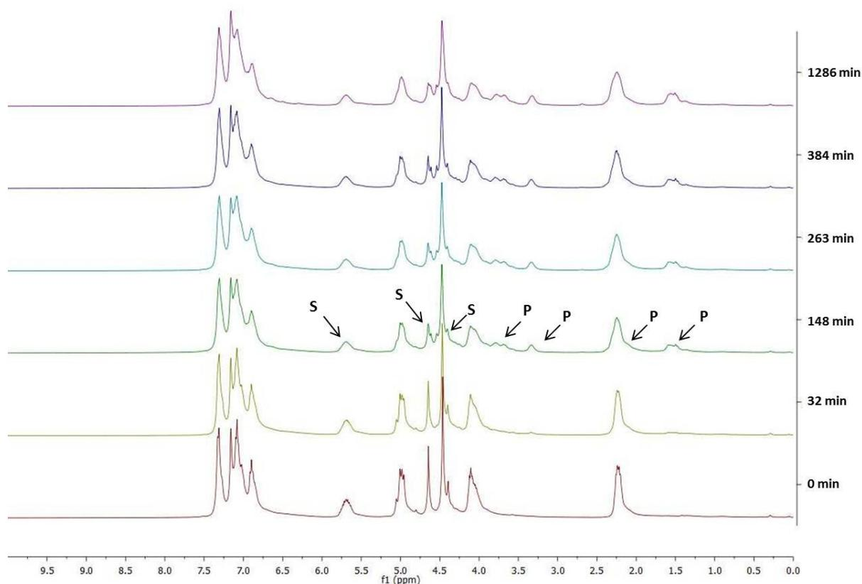
**Figure 20:** Overlay of the recorded  $^1\text{H}$  NMR spectra (S:  $[\text{CpCo(CO)}(\mathbf{30})]$  (**32**); P:  $[\text{CpCo}(\mathbf{30})]$  (**34**))
