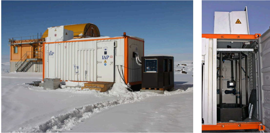
Figure 2.3.: Left: The Fe lidar container and chiller hut (black box on the right hand side of the container). The building housing the Australian lidar is visible in the background. Right: View of the telescope in the back of the container.
