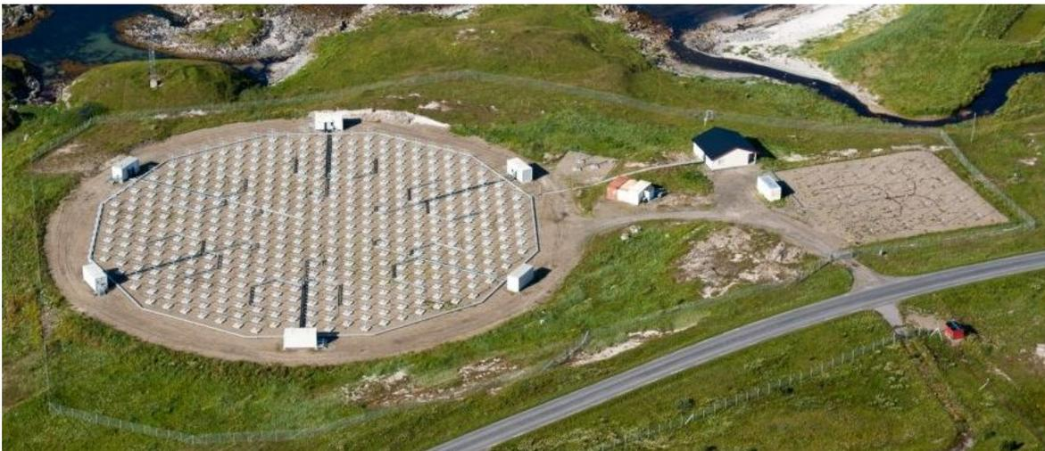
**Figure 1.1** Photograph of the MAARSY site, showing on the left the MAARSY antenna array, accompanied by the ALWIN64 antenna array on the right.
