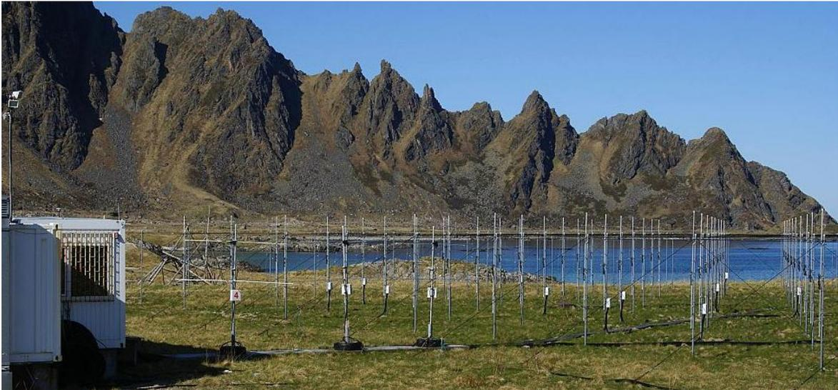
**Figure 3.1** Photograph of the former ALWIN radar. The container in the left housed the radar equipment, while a part of the 144 4-element Yagi array is shown on the right.
