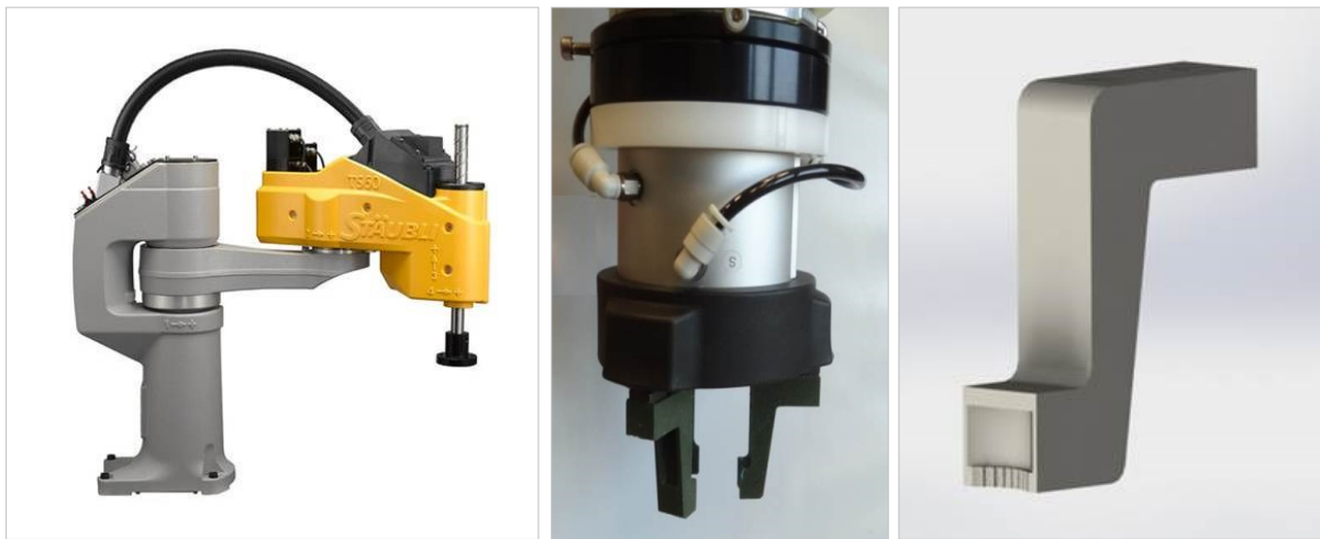
Fig 23: Stäubli® TS60 SCARA robot (left), pneumatic end effector with flexible finger design (middle), one individual finger (right)
