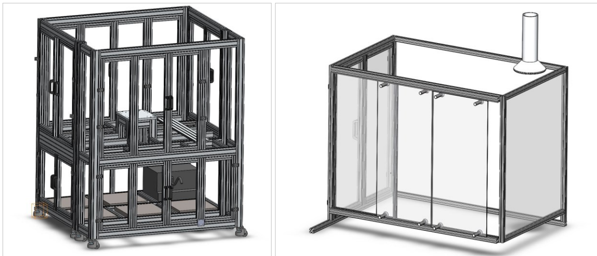
Fig 25: 3D CAD design of the housing for the TS60 SCARA robot assembly (left) and the housing for the Biomek® 2000
