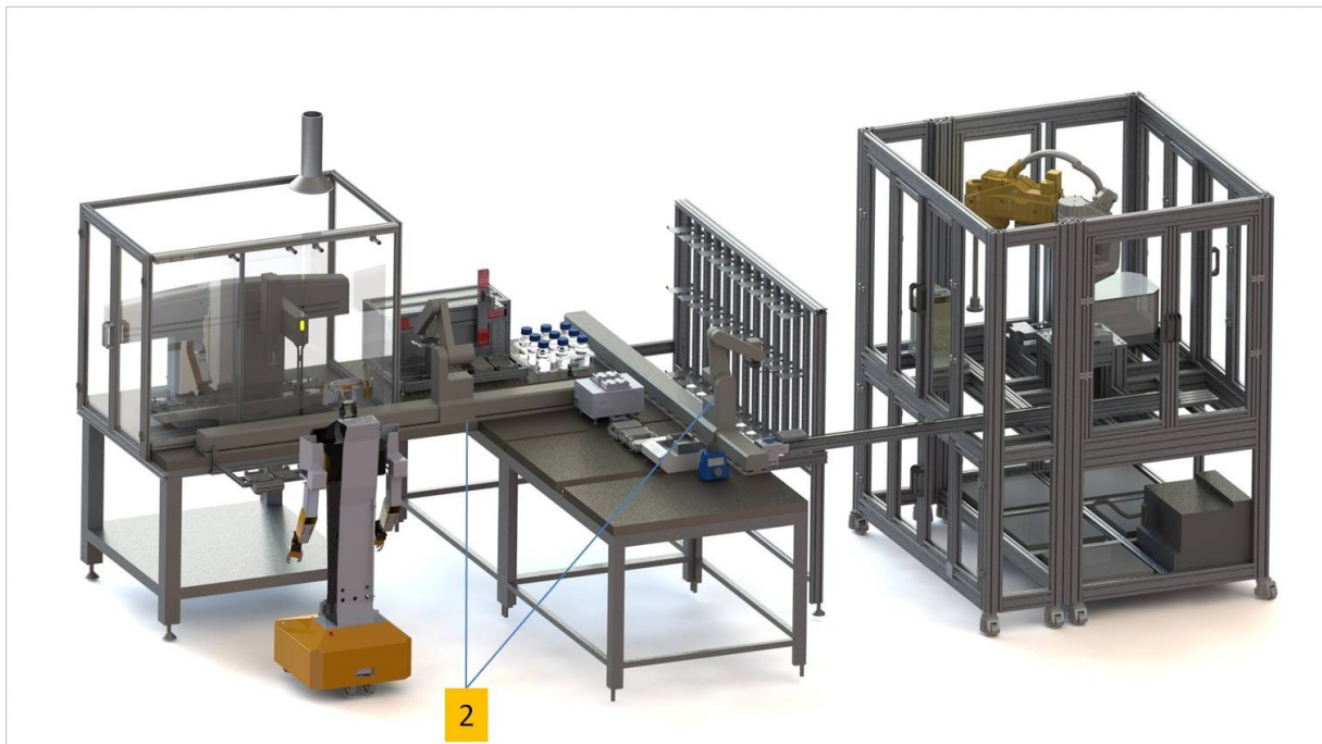
Fig 19: 3D CAD design of the automated system with two ORCAs® supplying system integration and sample transport
