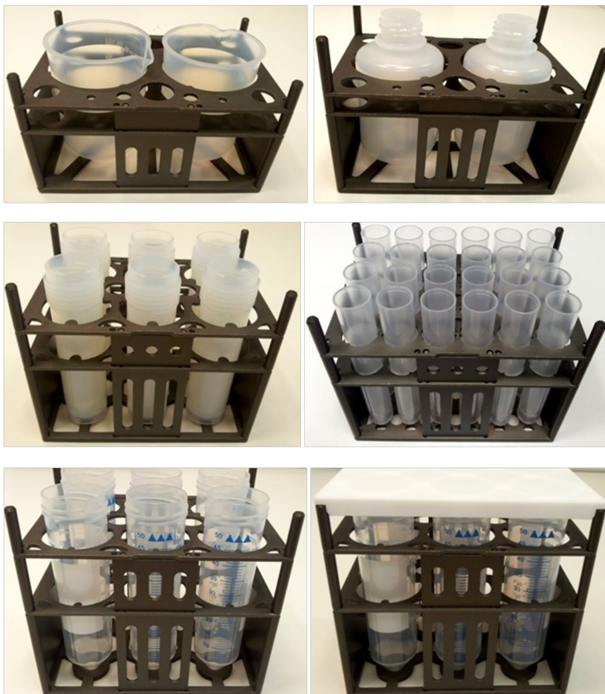
Fig 40: Conceived trays with embedded vessels for the automated mercury analysis process: (1) tray with two reservoirs for high concentrated acid, (2) tray with two reservoirs for water, (3) tray with six vessels for microwave digestion treatment, (4) tray with 24 calibration vessels, (5) tray with six analysis vessels, (6) tray with six analysis vessels covered by lid
