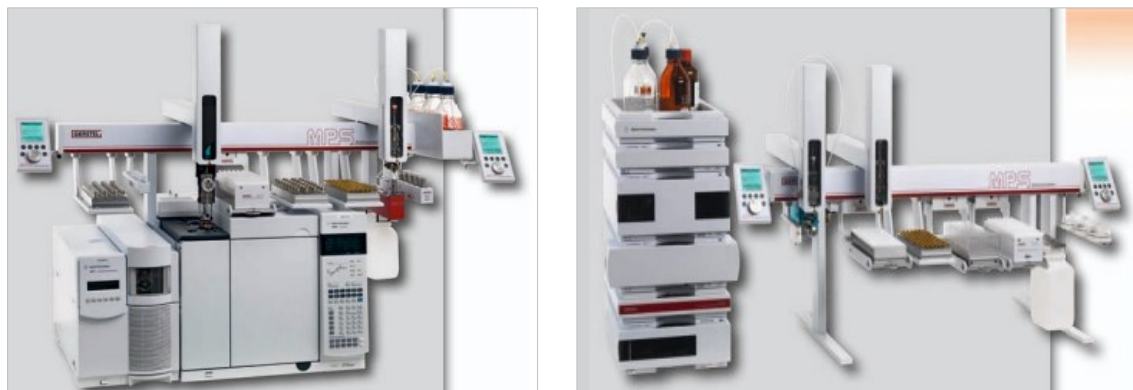
Fig 6: MPS Dual Head for automated sample introduction to a GC/MS and an HPLC system. Source: [v]
