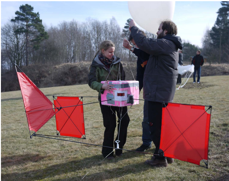
Figure 3.6: Photograph of the LITOS payload with three large windvanes, launched on 25th February 2011 from Kühlungsborn
