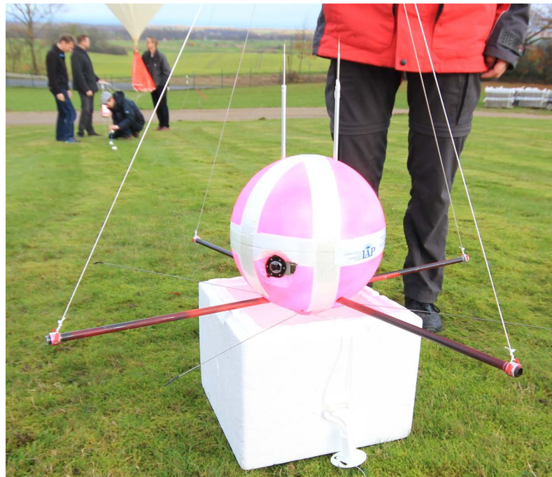
Figure 3.7: Photograph of the spherical LITOS payload launched on 20th November 2014 from Kühlungsborn. The cubic styrofoam box is not part of the payload, but is used for handling on the ground.
