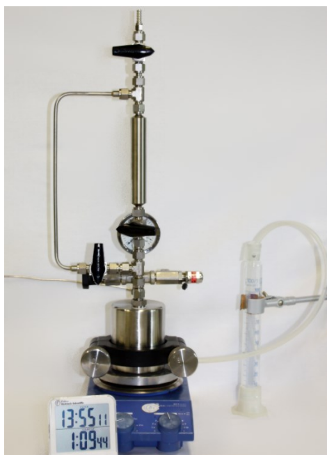
Figure A2-1. a) Dead-End Filtration Cell. b) Flow-Scheme: 1 – Refill reservoir, 2 – Feed stream, 3 – Permeate stream, 4 – Stirrer, 5 – Retentate stream, 6 – Magnetic stirrer.
