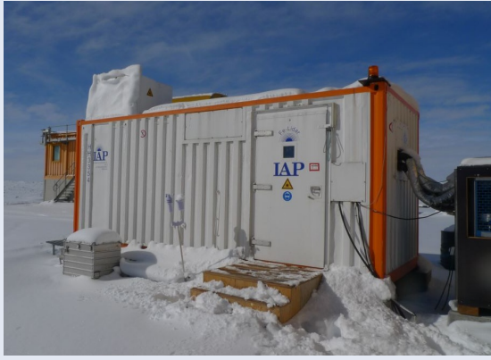
Figure 7: The mobile IAP Fe lidar at Davis, Antarctica (69°S) in March 2011. The system is housed in a single insulated 20' container, designed to be transported to remote polar regions. CC BY-NC 4.0
