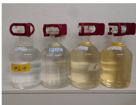
Figure 2.2: Artificial seawater samples spiked with humic acid (from left to right: 0, 100, 250 and 500 \mu\text{mol C/L} ).
