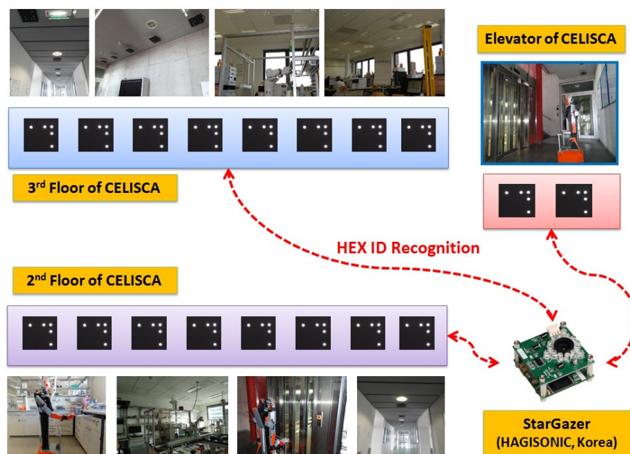
Figure 3-2: Mobile robot multi-floor navigation mapping strategy
