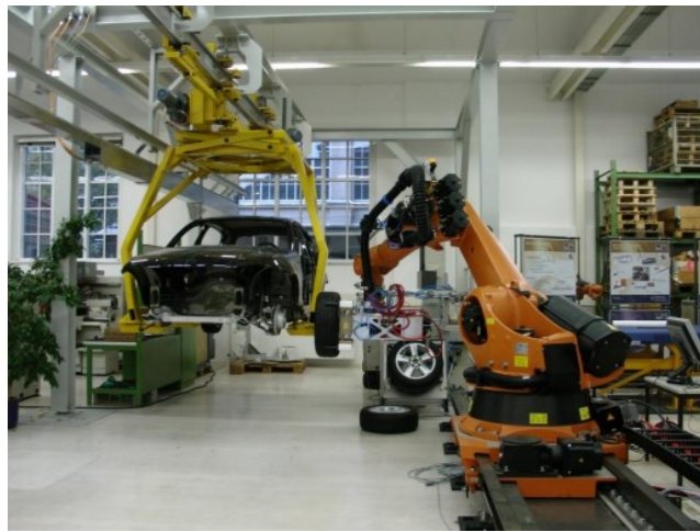
Figure 1-2: Car-wheel assembling and transporting robotic system [23]
