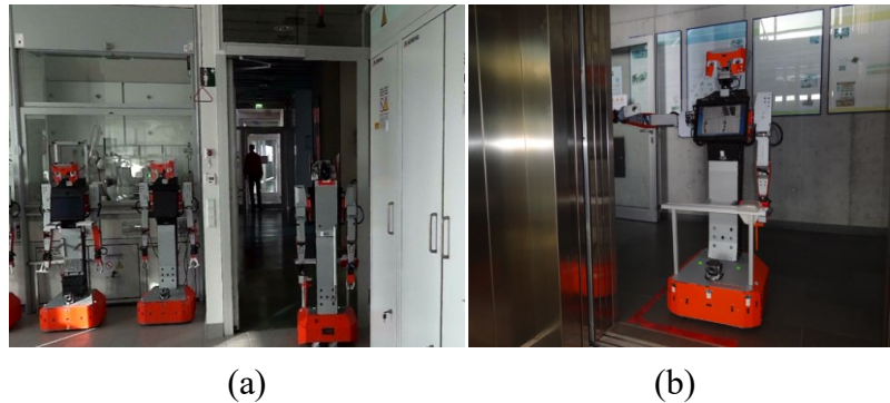
Figure 3-5: Laboratory door-opening/closing by the running mobile robots: (a) Automatic controlling for the laboratory doors; and (b) Automatic controlling for the elevator doors
