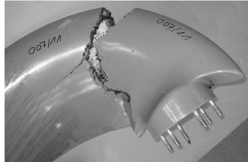
Figure 1.2: Permanent failure of the mixer blade while application [14]
