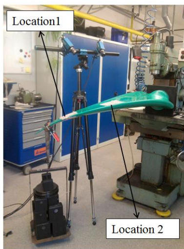
Figure 5.6: Vic 3D camera setup for the experiment
