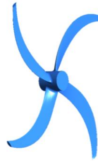
Figure 4.2: CAD model of the tidal-turbine blade provided by SCHOTTEL GmbH
