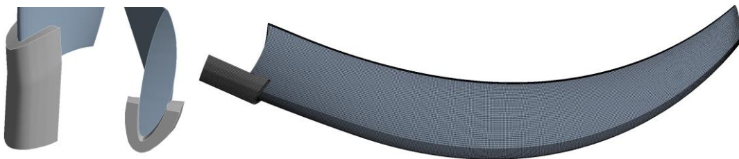
Figure 7.3: U-Profile connector added at the hub end of the blade. Cross-sectional view of connector (left) and mesh topology (right) are shown [82].
