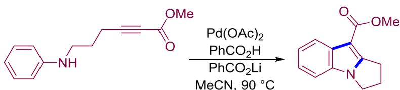
**Scheme 51:** Example of palladium-catalyzed domino reaction involving intramolecular hydroamination<sup>[161]</sup>
