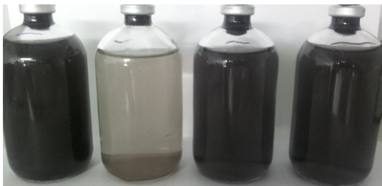
Figure 6: Dilution to extinction series with \text{MnO}_2 and \text{S}_2\text{O}_3^{2-} to isolate S. marisnigri . From left to right: sterile control, dilution of 1:10^4 , dilution of 1:10^5 , and dilution of 1:10^6 from the previous culturing series.
