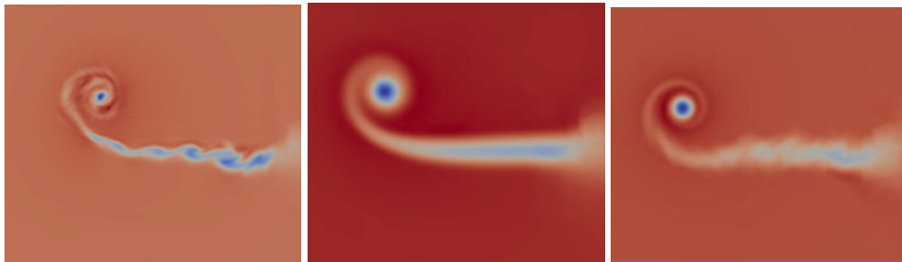
FIGURE 7.37: Velocity iso-surfaces at x/c = 5 . Left : w/o Turb. model, Middle : SST model Right : LES model
