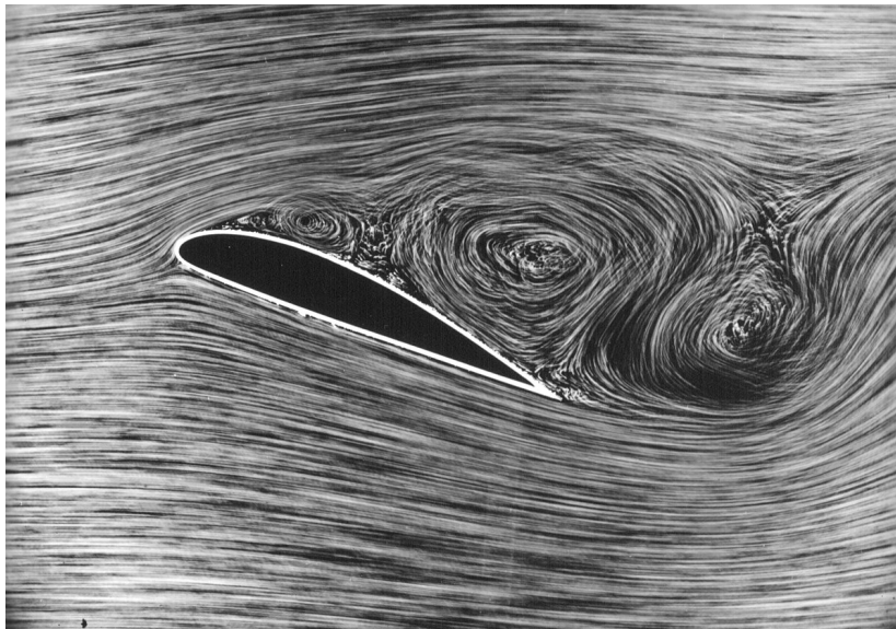
FIGURE 4.1: Photograph of a airfoil in a wind tunnel, showing flow separation over the top surface. Taken by DLR in 1915.
