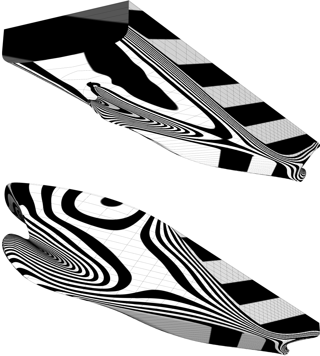
Figure A.2.: Reflection analysis of the generalized B-spline surface.
