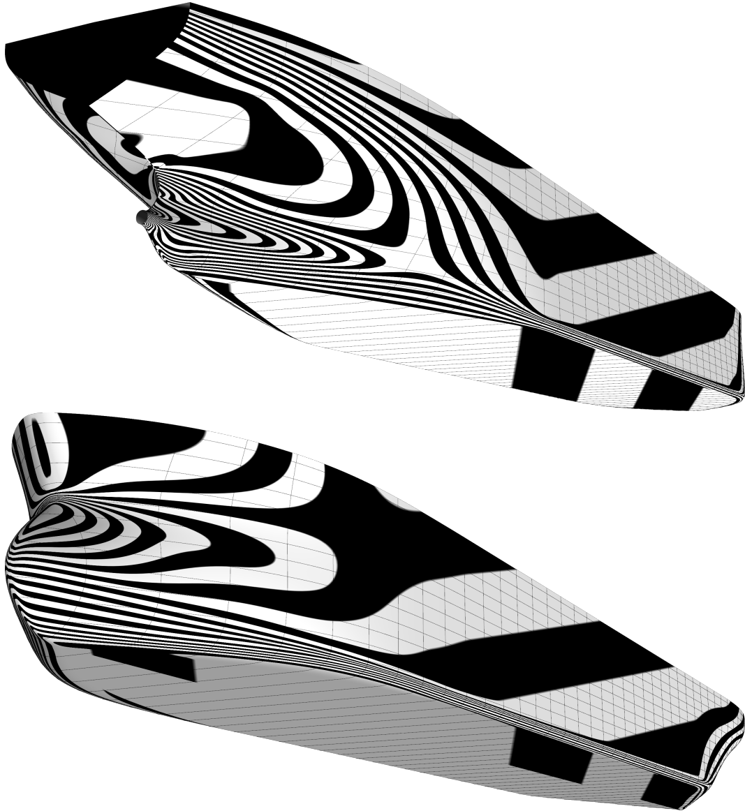
Figure B.2.: Reflection analysis of the generalized B-spline surface.
