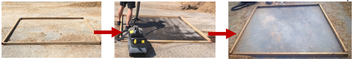
Fig. 9: Cleaning method of the grid square with a wet vacuum cleaner before, during and after cleaning
