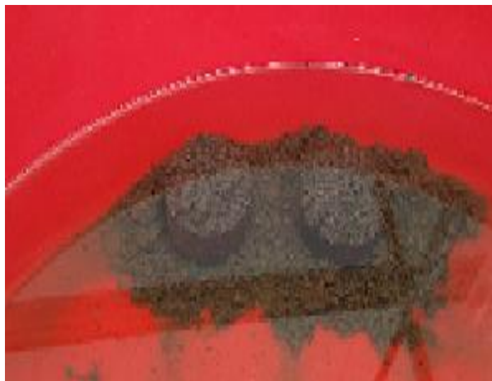
Figure 4.21: The BC soil samples failed in the first cycle
