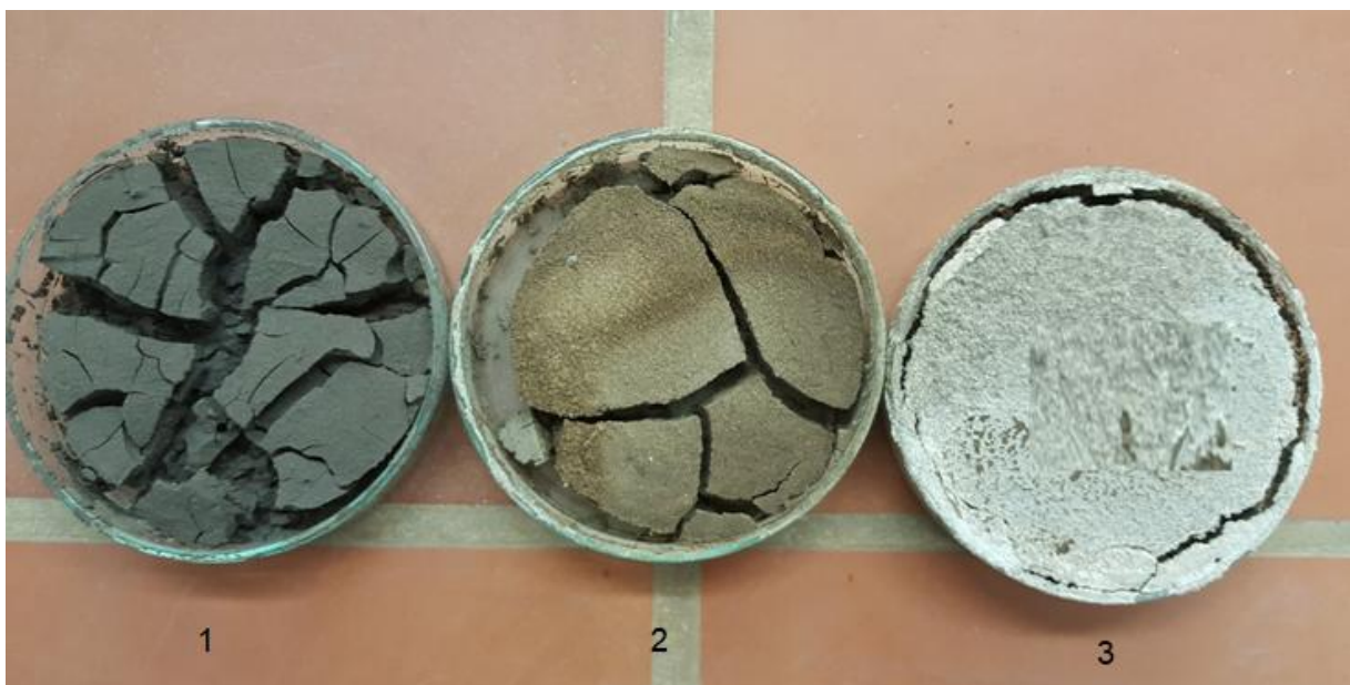
Figure 4.7: Shrinkage behaviour (1) BC soil, (2) 10% CHA and (3) 20% CHA
