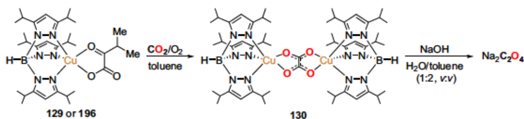
Scheme 73: Reaction of complex 129 or its ^{13}\text{C} -labeled analogue 196 with \text{CO}_2/\text{O}_2 (~1:1) in toluene and subsequent removal of oxalate with NaOH.
