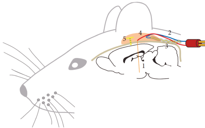
Figure 1.5: Schematic depiction of a DBS setup in rats. 1 – DBS electrode, 2 – cables to connect to the pulse generator, 3 – grounding gold wire (note that it is placed outside of the skull), 4 – acrylic mounting, 5 – fixating screw that can be used for grounding. The image is adapted from [47].
