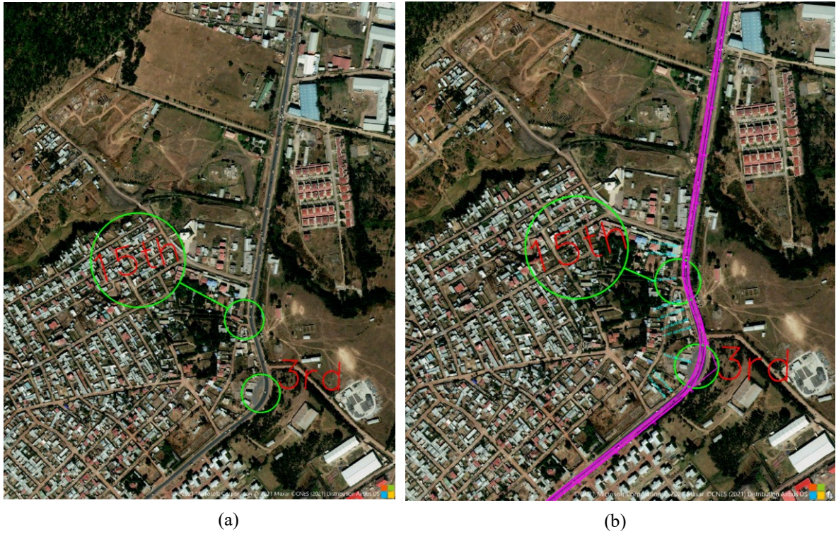
Figure 20: (a) the existing road at the third-ranked hazardous road segment; (b) re-designed
