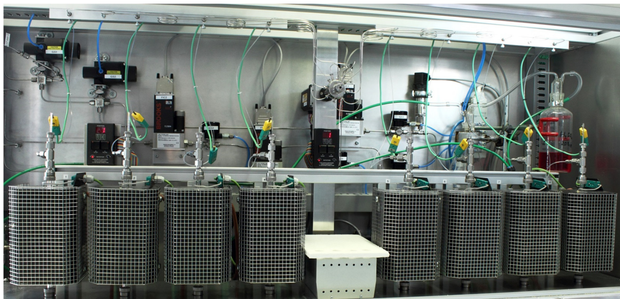
Figure A-1 A graph photo of in-house developed setup with eight continuous-flow fixed-bed quartz reactors for H_2 -TPP, CO_2/CO -TPD, and TPH tests.
