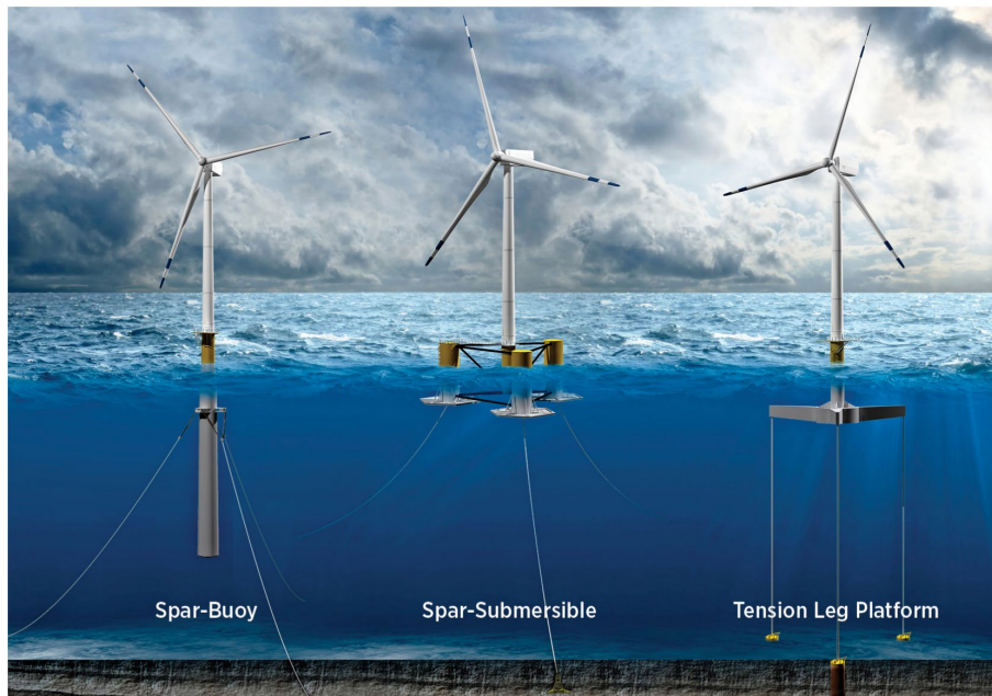
FIGURE 6: FLOATING OFFSHORE WIND TURBINE SUBSTRUCTURE CONCEPTS (GRAPHIC BY JOSH BAUER, NREL)
