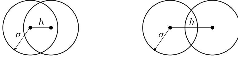
(a) h < \sigma , overlap criterion has been fulfilled (b) h > \sigma , overlap criterion has been broken
