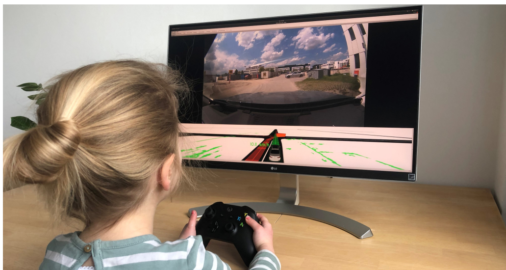
Figure 4.1: Image of the operator workplace: A human operator controls the vehicle using a gamepad.
