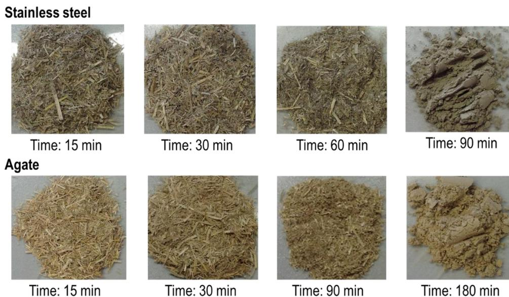
**Figure 14.** Grinding rice straw in the ball mill with different conditions
