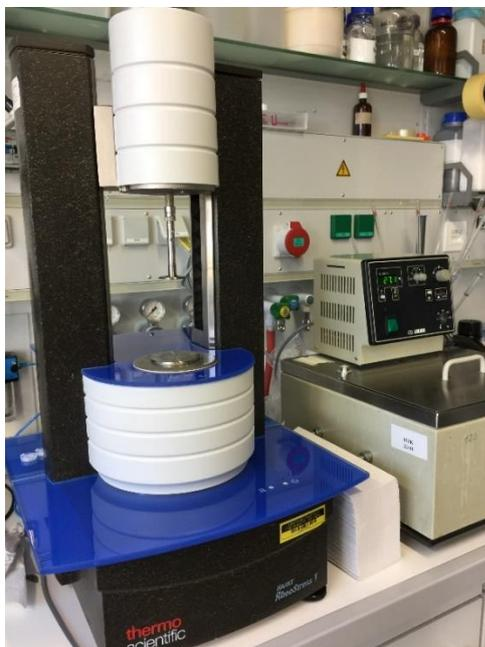
**Figure 83.** Viscosity equipment Rheo Stress 1 Thermo Scientific Haake
