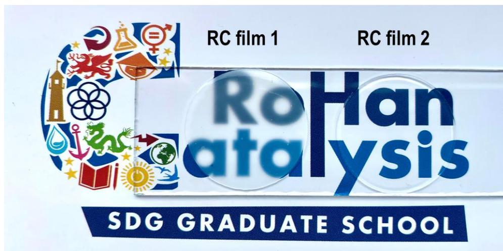
**Figure 47.** RC film 1 (without DMSO), left and RC film 2 (with DMSO), right
