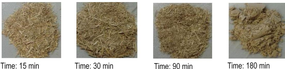
**Figure 81.** Grinding rice straw by the planetary ball mill with different time
