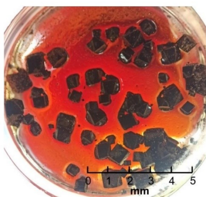
Figure 7. Microscopic view of crystals of 1 under 20-fold magnification.
