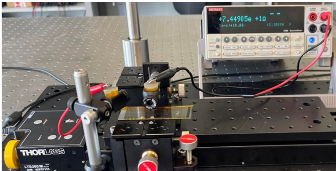
Figure 4.1: Custom assembled setup for measurement of electrical resistance of approximately 60 \mu\text{m} wide and 600 nm thick gold microelectrode using probe needles.
