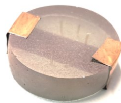
Figure 2.19: Sample preparation for obtaining a cross-section image of optical fiber using SEM.
