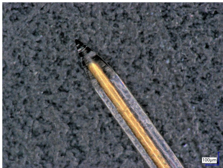
Figure 2.21: Microscope image of gold microelectrode deposited on cone tip of the optical fiber.
