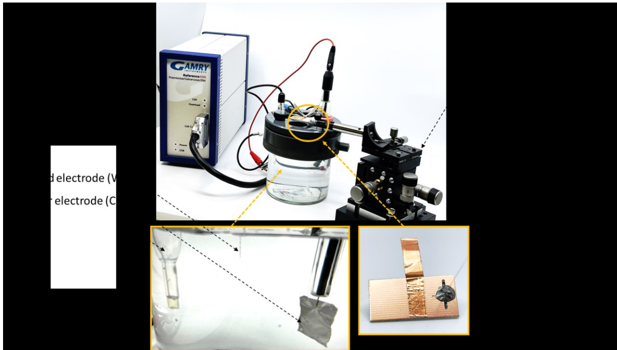
Figure 4.7: Measurement setup (3-electrode setup) for electrochemical impedance of recording electrode fabricated in this work. Working electrode and working sensing leads are both connected to tested electrode (WE). Counter electrode is connected to 99.99% platinum electrode, while reference electrode and reference sensing are both connected to an encapsulated Ag/AgCl wire.
