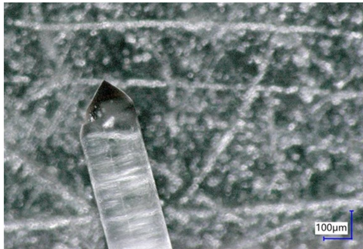
Figure 2.11: Optical fiber with asymmetric cone shape, created using mechanical grinding setup, caused by misalignment of the optical fiber in the V-groove of fiber rotator.
