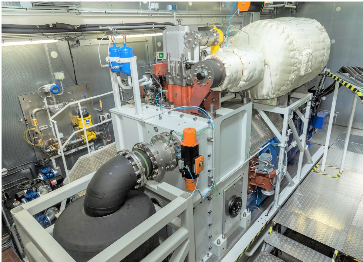
Figure 3.1: Dual-fuel research engine at Rostock University.
