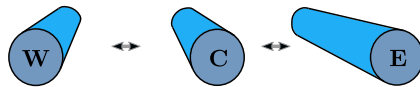
Figure 10.: Elementary architecture for the generation of nonadiabatic holonomies. The distances between the outer modes W and E, and the central one C determine the coupling.
