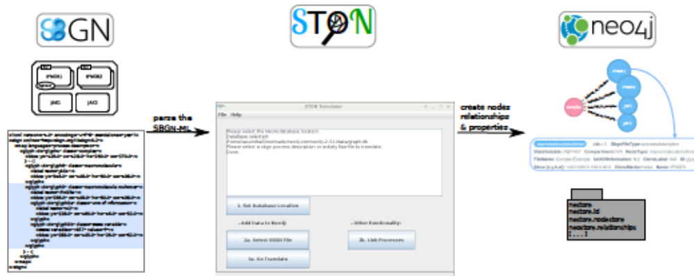
Figure 8.9.: Workflow of the STON framework [Touré et al., 2016] : an SBGN-ML file is provided as the input to the framework. It is parsed by STON and converted into a graph representation using mapping rules. The resulting data is then stored in a local directory as nodes, relationships and properties. Neo4j relies on this repository and, if run as a web server instance, offers a visualization of the data. The repository can be queried for biological entities, relations in the network, and similar nodes across networks.
