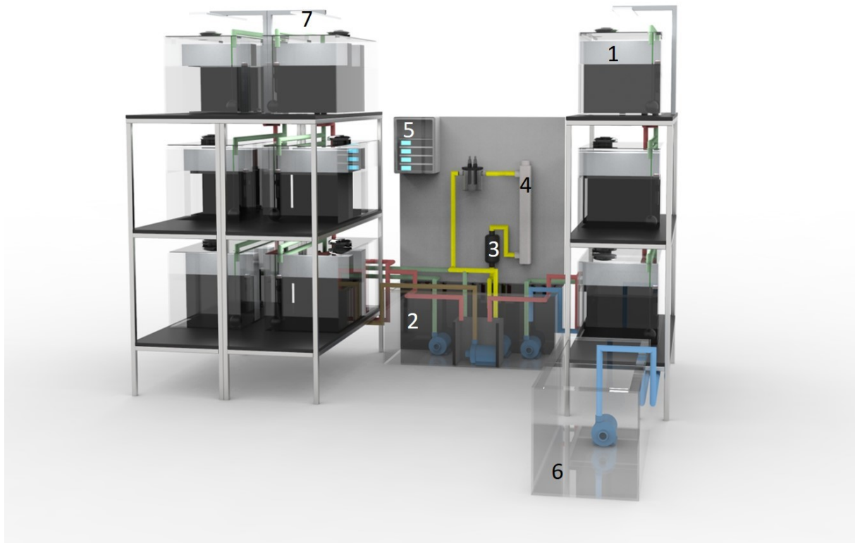
Figure 3.1: Overview of the experimental recirculating aquaculture system. 1. Aquarium, 2. Sump with pumps and solid separation compartment, 3. Flow through heater, 4. UV-C light, 5. Computer to control the light and water exchanges, 6. Separate aquarium for water exchange, 7. Light bar.
