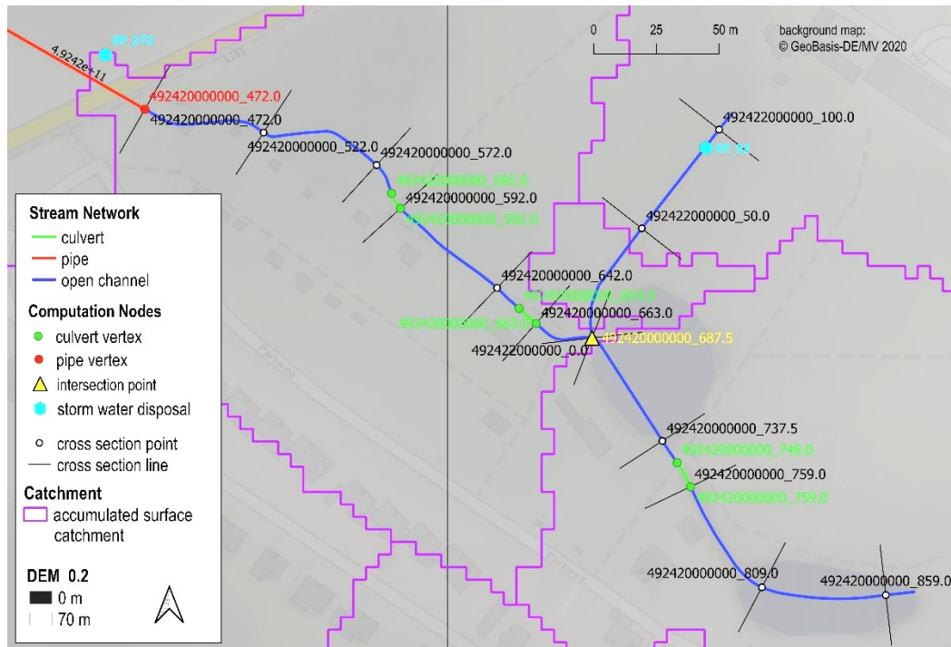
Figure 17. Calculation nodes of the stream network composed of pipe and culvert vertices, cross sections points, intersection points, and storm water disposals (DEM_0.2 = digital elevation model with a cell size of 0.2m).
